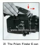
be attached to the camera body very easily, too. First, place the protrusions on the bottom of the finder into corresponding openings in the finder frame and, then, slide the finder forward until it locks.
