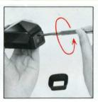
2) To exchange the eyepiece lens, first, detach the eyecup. Then, unscrew the setscrew on the eyepiece lens frame which will permit the lens to be removed together with its frame.
